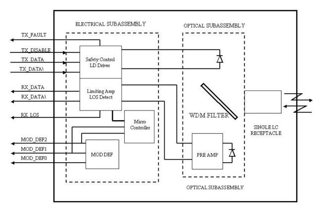
**Transmitter Section-** The Laser driver accept differential input data and provide bias and modulation currents for driving a laser. An automatic power-control (APC) feedback loop is incorporated to maintain a constant average optical power.1310 DFB in an eye safe optical subassembly (OSA) mates to the fiber cable.
